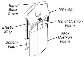
FIGURE 1 - REMOVING/INSTALLING BACK CUSHION FOAM
